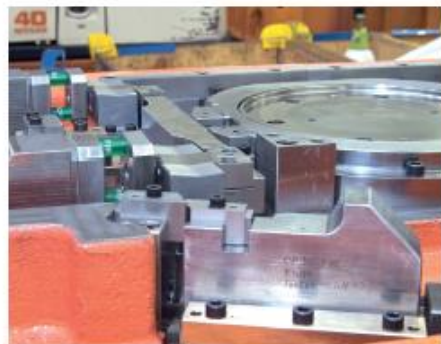
Pic.1: Washing machine die.
