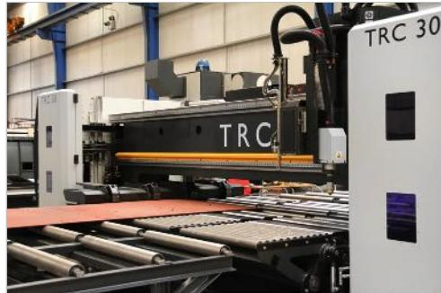
Machine front for thermal cutting
