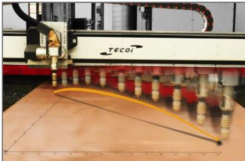
The IMZ® (intelligent movement Z-axis) system reduces the time of the cutting process by up to 30% allowing faster and more accurate head positioning in the Z-axis. Furthermore, the IMZ® system increases productivity by up to 70% in between piercings.
