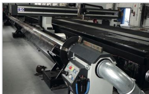
Tube cutting with servo-controlled rotation Corte de tubos con giro servo-controlado
