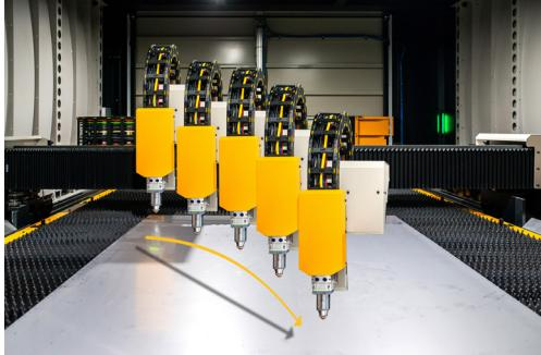
The IMZ® (intelligent movement Z-axis) system reduces the time of the cutting process by up to 30% allowing faster and more accurate positioning of the head in the Z-axis. Furthermore, the IMZ® system increases productivity by up to 70% in between piercings.
