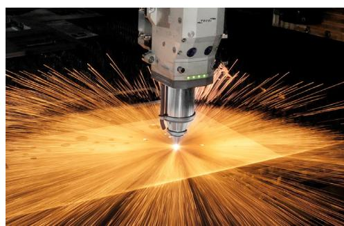
The controlled piercing system SPC® increases the plasma, oxy-fuel and laser piercing capacity, effectively raising the maximum cutting thickness and lifespan of the consumables by up to 25% and 30% respectively.
