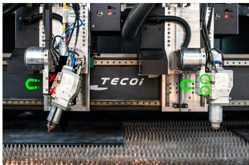
Three-dimensional anti-collision system with automatic high speed resets that provide the plasma, oxyfuel and laser torches with increased safety (SAC-L®) while guaranteeing accurate positioning during straight and bevel cutting operations.
