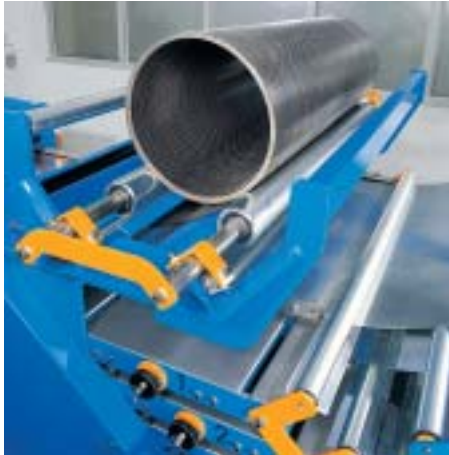
ARG-MT deroller assembled on a coil selector
