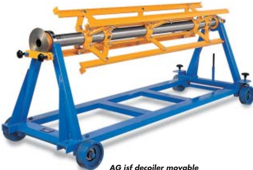
AG isf decoiler movable with expanding diameter shaft up to 5 tons coil weight and 2000 mm coil width
