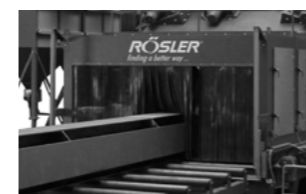
Roller conveyor blast machine for weldments
