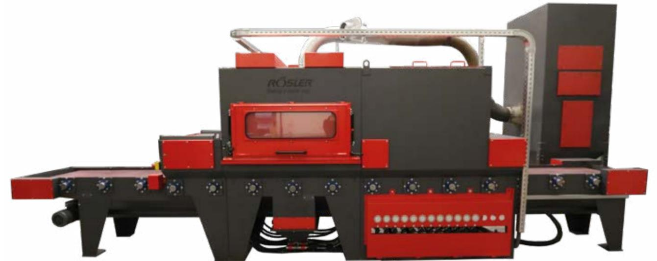
Continuous feed belt blast machines are used for cleaning, stripping and surface preparation prior to bonding or coating tasks in continuous feed operations. They are ideal for continuous manufacturing operations with relatively high work piece volumes. Practically no productive time is lost through work piece loading and unloading. The blast media is always thrown from above the belt. Oscillating movement of the blast nozzle(s) ensures optimum blast coverage.
