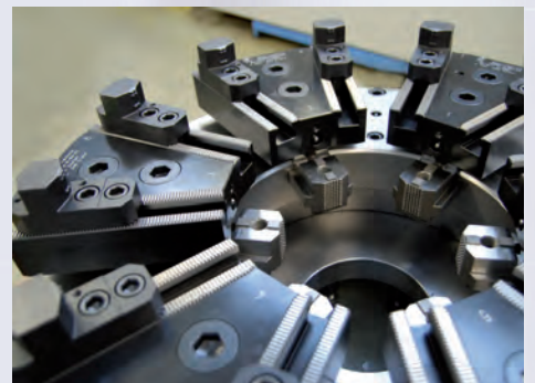
Variable positioning of the clamping jaws on the pendulum segments
