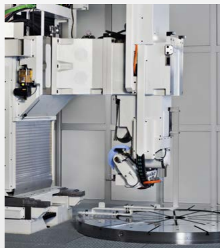
ZP E/I with changeover between external and internal machining that does not require set-up
