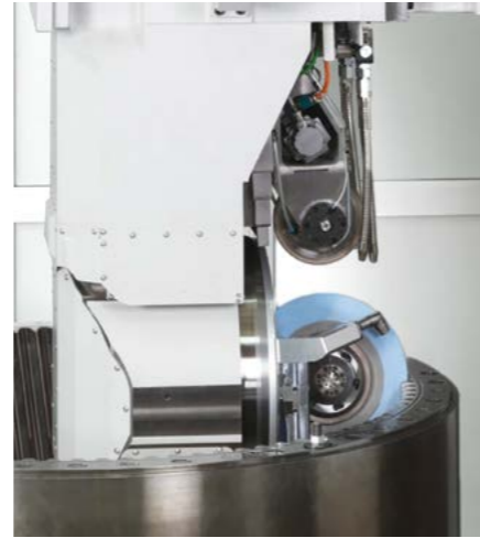
ZP I/E with grinding arm that can be swivelled quickly for machining internal and external gears with large modules and gear widths
