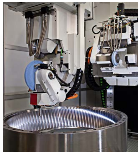
ZP E/I with changeover between external and internal machining that does not require set-up
