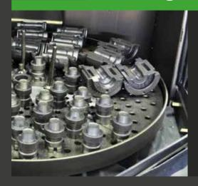
POMETON GRANINOX Stainless steel shot is highly recommended when the chemical and color contamination typical of standard high carbon steel blasting cannot be accepted.
