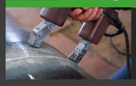
Thanks to their magnetic behaviour POMETON FERILEV iron powder is ideal in a number of magnetic applications, like non-destructive magnetic tests (i.e. on welding and casting discontinuity). This process permits to identify possible cracks or defects without damage the component.
