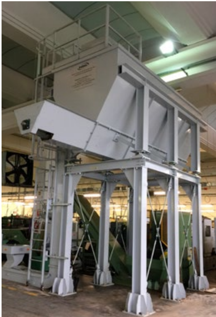
Horizontal silos equipped with load cells
