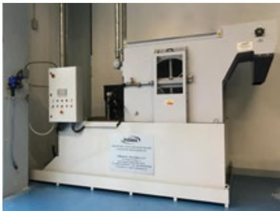
Self-cleaning unit for both neat oil and emulsion
