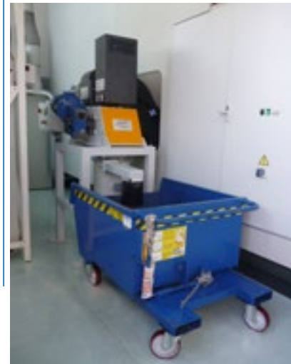
Shredding and spinning unit under the machine tool conveyor
