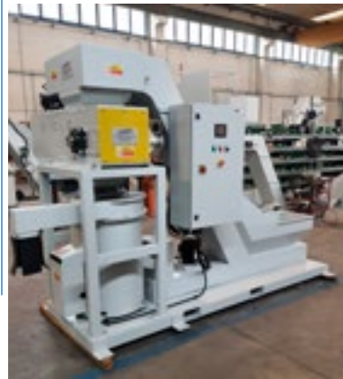
Grinder and centrifuge fed by a conveyor
