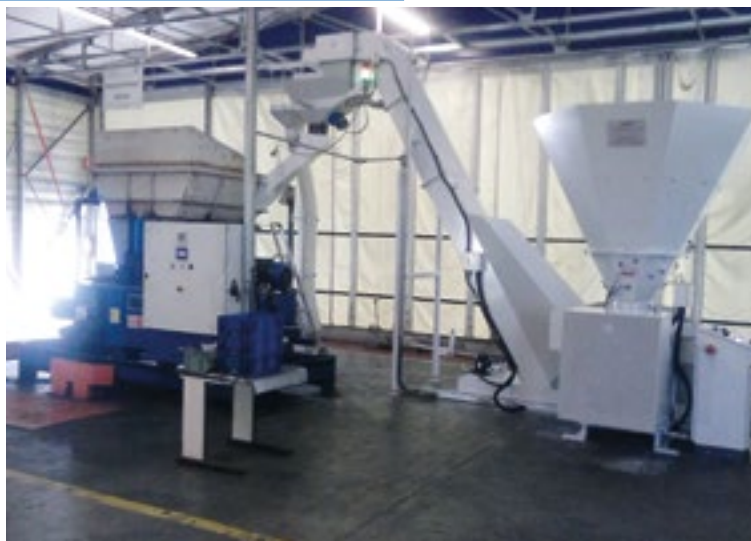
Automatic crushing and briquetting system
