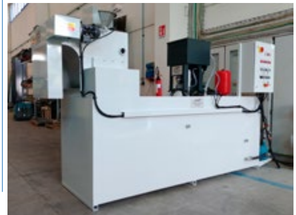
Self-cleaning unit for both neat oil and emulsion
