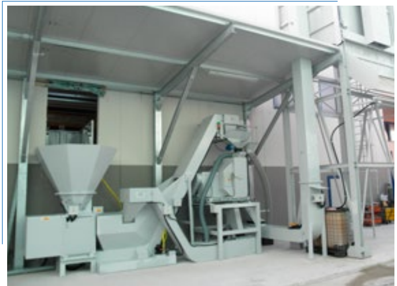
Swarf crushing and spinning plant with silos
