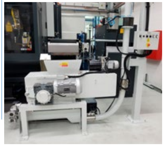
Vacuum station equipped with grinder
