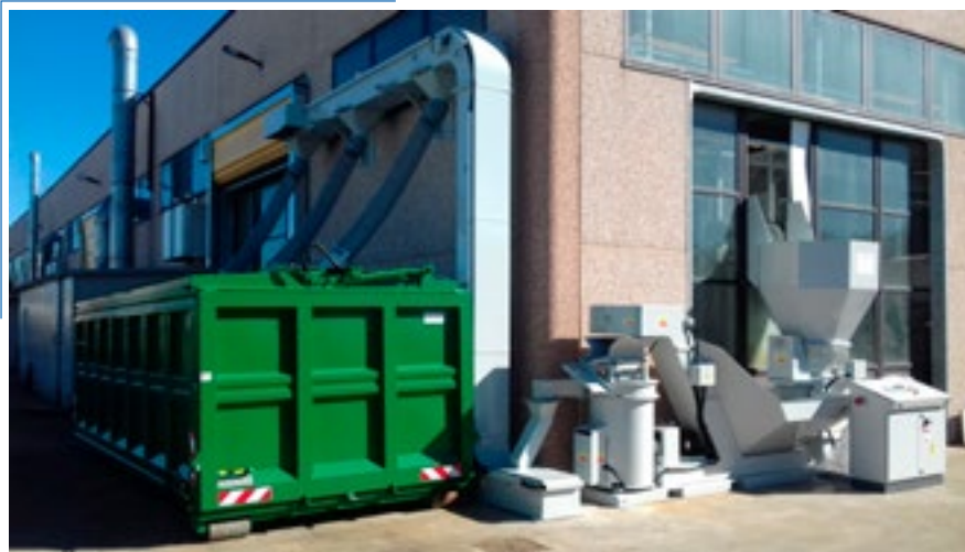
Minisystem with crusher and automatic discharge into a container
