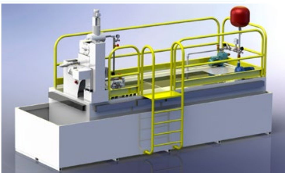
Centralized unit to filter and top up the machine tools
