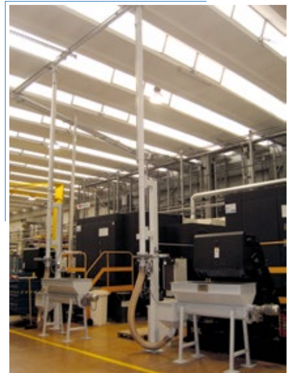
Vacuum station for fine aluminium swarf
