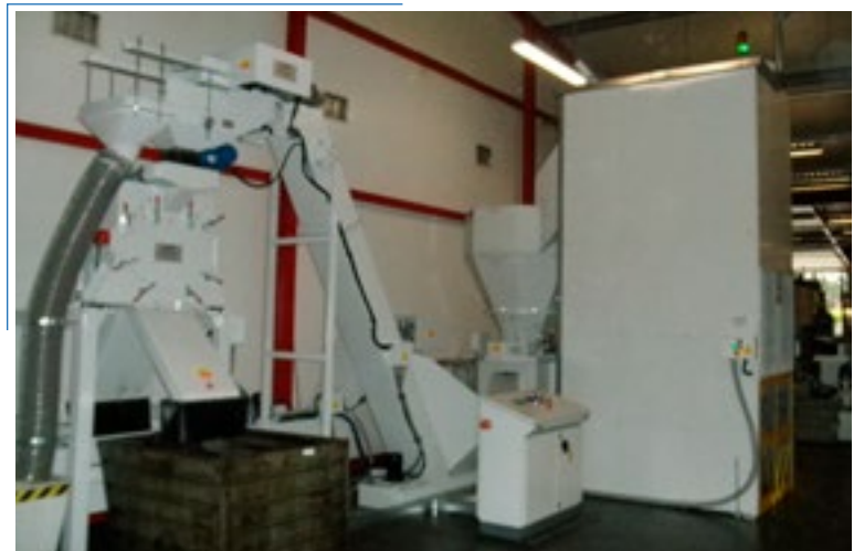
Automatic crushing and spinning system equipped with skiphoist
