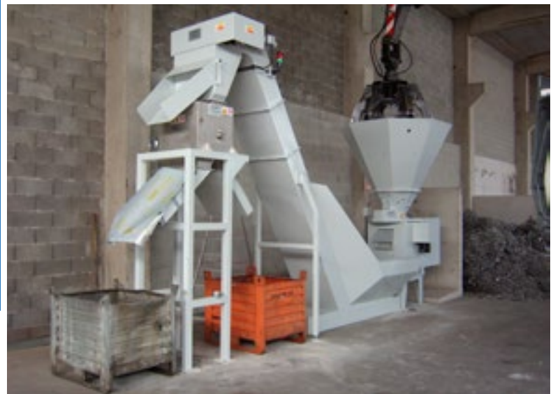
Automatic crushing system equipped with magnetic separator
