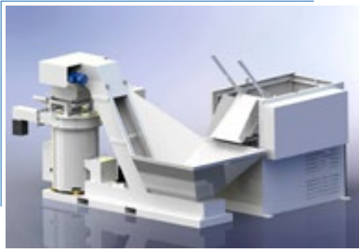
Minisystem with skipoist and 800 Lt conveyor hopper volume
