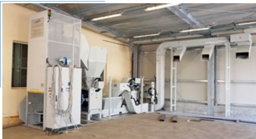
Minisystem with skiphoist, crusher and discharge into container
