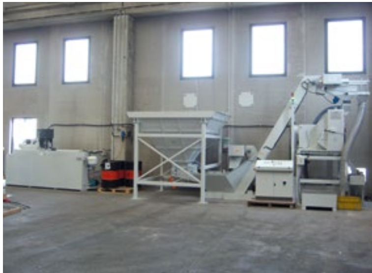
Automatic spinning plant with 6m3 pre-storage hopper
