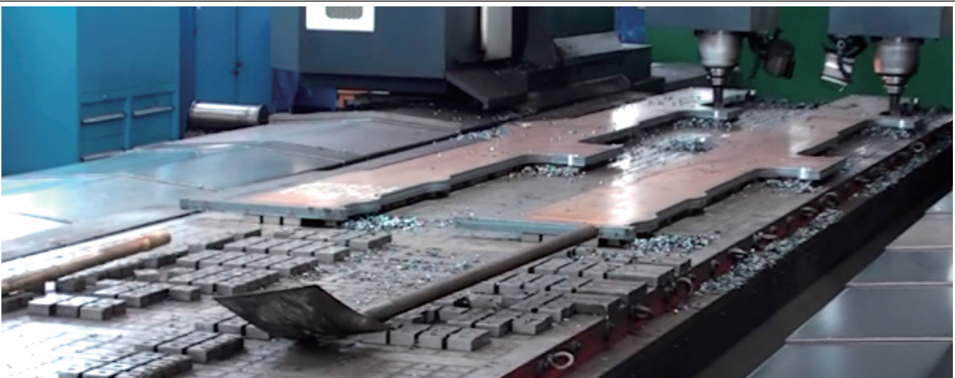
Used on Double Column Machining Center for machining big & multi-medium workpiece 5 sides machining.
