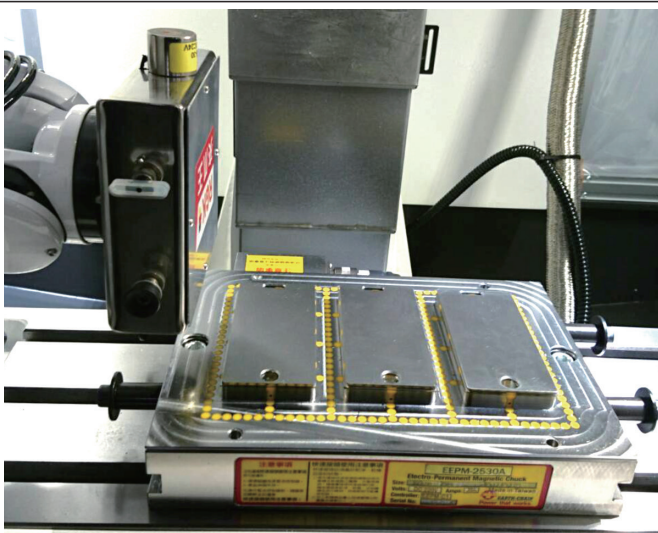
Used for cell phone case fine grinding.
