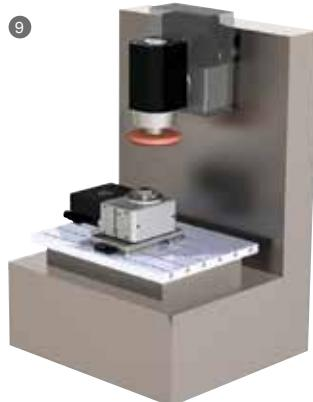
4th axis for tilting the grinding spindle.
