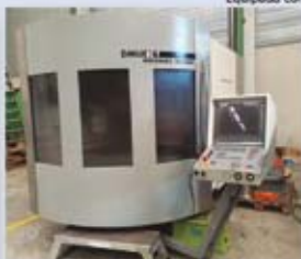
Centro DECKEL MAHO DMU 80 T 5 E3ES HEIDENHAIN TNC430 recorridos 880-630-630 mm.
