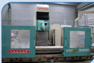
Fresadora de bancada fija ANAYAK VH Plus 3000N cnc HEIDENHAIN HEIDENHAIN TNC-407 recorridos 2000x500x500 mm
