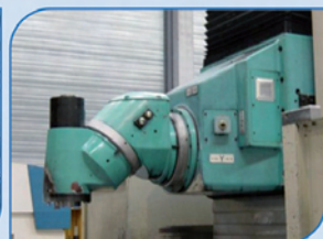
Fresadora de bancada fija ANAYAK VH Plus 3000N cnc HEIDENHAIN HEIDENHAIN TNC-407 recorridos 2000x500x500 mm
