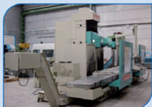
Fresadora de bancada fija ANAYAK VH Plus 3000N cnc HEIDENHAIN HEIDENHAIN TNC-407 recorridos 2000x500x500 mm
