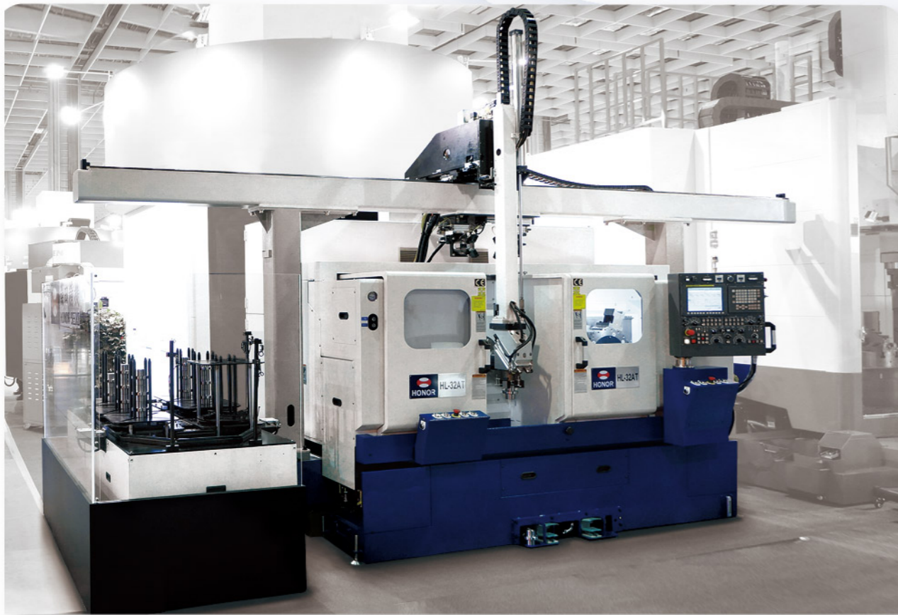
■ Type1 : Single loader Left side loading/unloading
